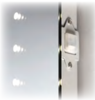
Rocker Switch to activate LED's
