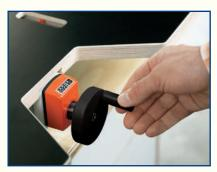
Practical and precise ruler system The drilling distance is set easily from the front using a calibrated spindle.
