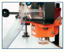
Insertion of Blum components MINIPRESS M is equally efficient when it comes to inserting Blum fittings. The operation is both simple and precise.
