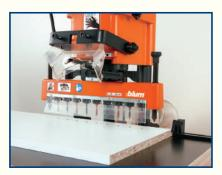
**9 spindle drilling head**For efficient drilling of hole groups within the 32mm system.
