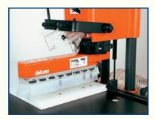
**8 spindle drilling head** For the assembly of BOX front fixings and cabinet profiles.
