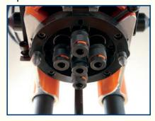
**Quick connect chuck**For quick and comfortable drill bit changeovers. The quick connect chucks can be retrofitted individually.
