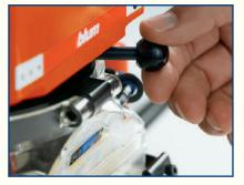
Drilling of various patterns With the multi-swivel drilling head, various drilling patterns for furniture fixings can be set quickly, precisely and without the need for tools.
