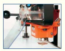
**Insertion of Blum components** MINIPRESS P is equally efficient when it comes to inserting Blum fittings. The operation is both simple and precise.
