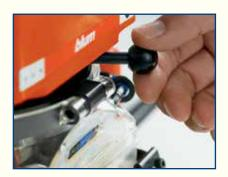
**Drilling of various patterns**With the multi-swivel drilling head, various drilling patterns for furniture fixings can be set quickly, precisely and without the need for tools.
