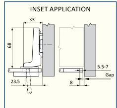
For glass thicknesses from 4.5 to 7 mm no gap is required.
