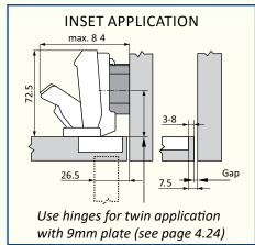
For fronts up to 21 mm thick, no gap is required. A trial is recommended for door thicknesses greater than 22 mm.
