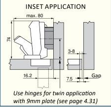
For fronts up to 24 mm thick, no gap is required. A trial is recommended for door thicknesses greater than 24 mm (22 mm where a boss drilling distance of 7 mm or greater is used) or for an overlay application against a wall.
