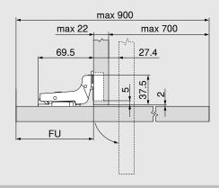
Hinge dimensions based on factory setting (mounting plate spacing = 0 mm)
