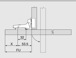
Fixing position cruciform mounting plate with dimension 37/32
