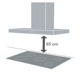
The hood is to be installed at a minimum distance of 65 cm from the cooking top, except for particular models where is specified in the technical drawing and instructions manual.
