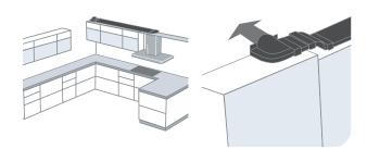
The position and distance of the exit hole (very long and very curved right-angled tubes limit hood efficiency).
